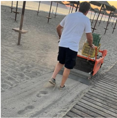
Photo 8 Usage of sand leveling machine. (Chania, July 2022)
